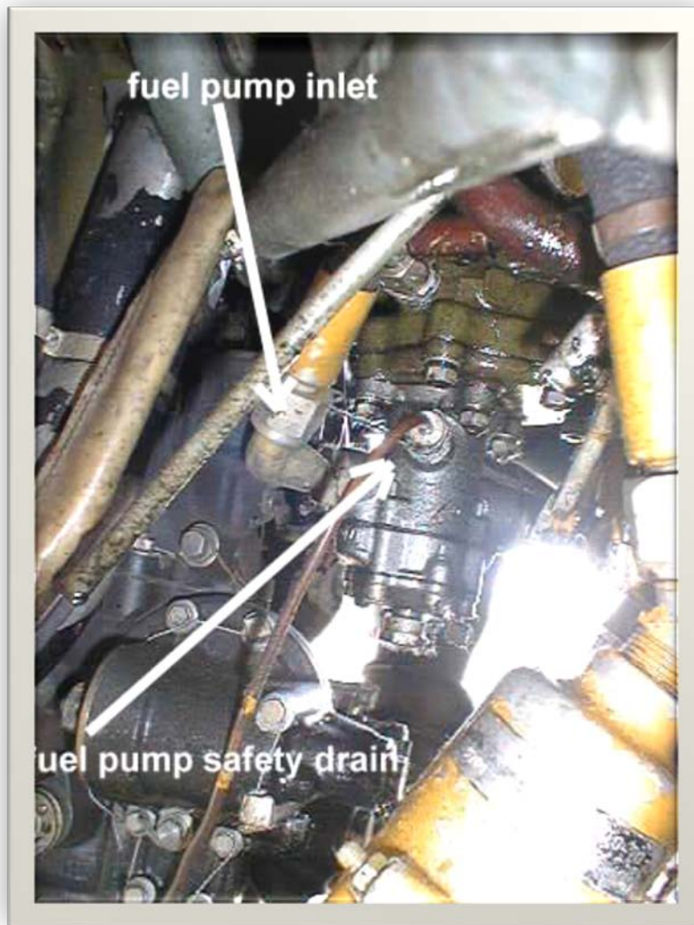
Figure 6. Fuel Pump Inlet (Fuel Pump Inlet Fitting P/N 526200-2W)
