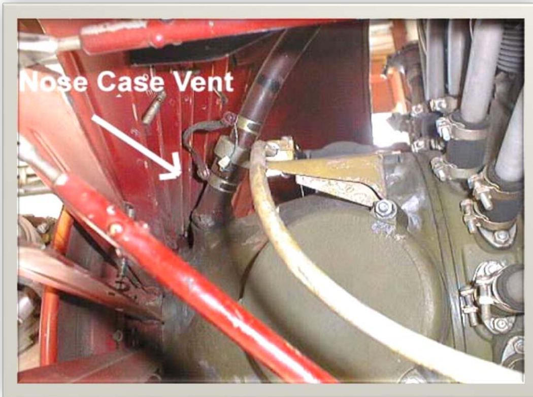
Figure 3. Nose Case Vent (Oil Breather/Vent Nose Case P/N 526200-120W)
