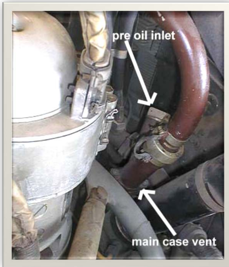
Figure 4. Main Case Vent (Oil Breather/Vent Main Case P/N 526200-100W)
