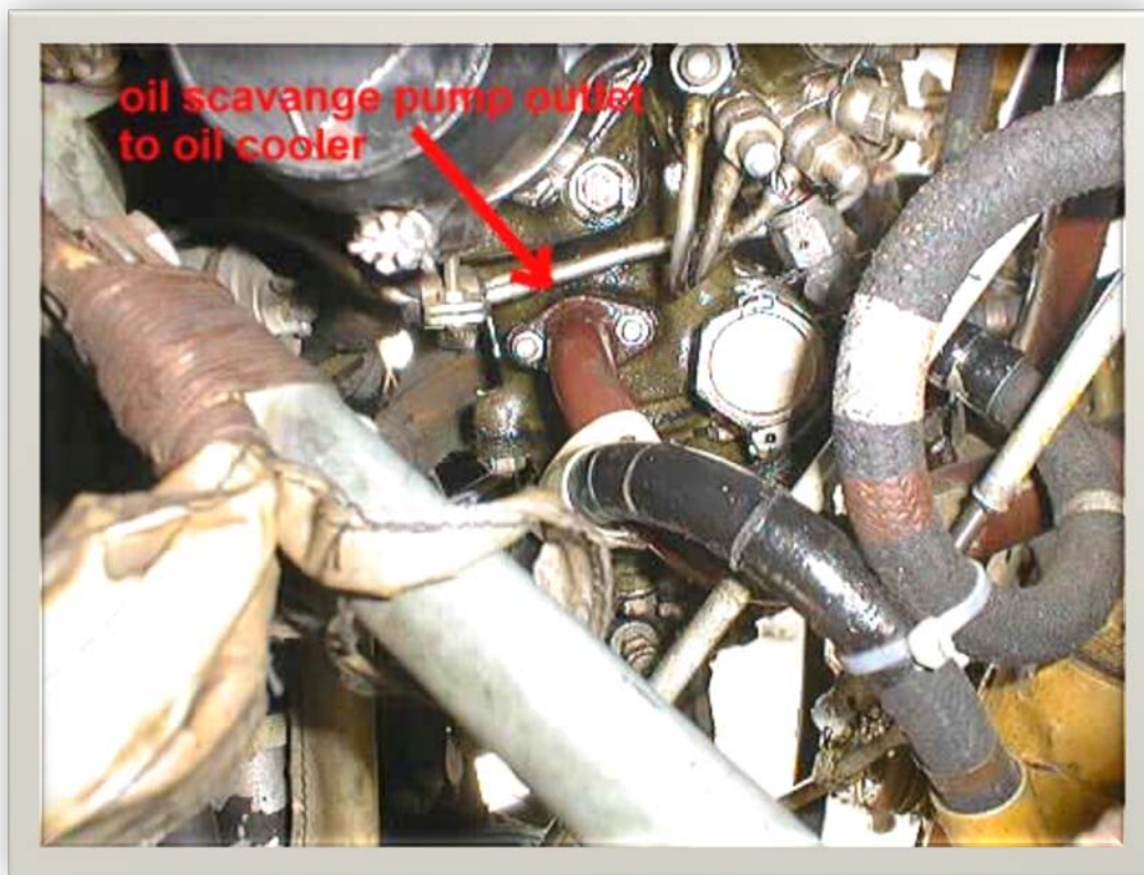
Figure 2. Oil Scavenge Pump Outlet (Oil Scavenge Pump P/N 526200-10W)
