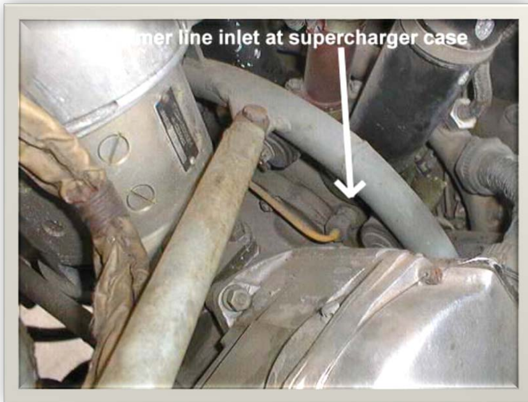
Figure 8. Primer Inlet To Supercharger Case (Primer Line Inlet Fitting P/N 14-717-107-01W)
